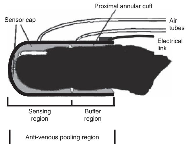
**Figure 4** Peripheral arterial tonometry finger probe. Cross-sectional image of digital pulse amplitude tonometry probe (image courtesy of Itamar Medical Ltd.).
