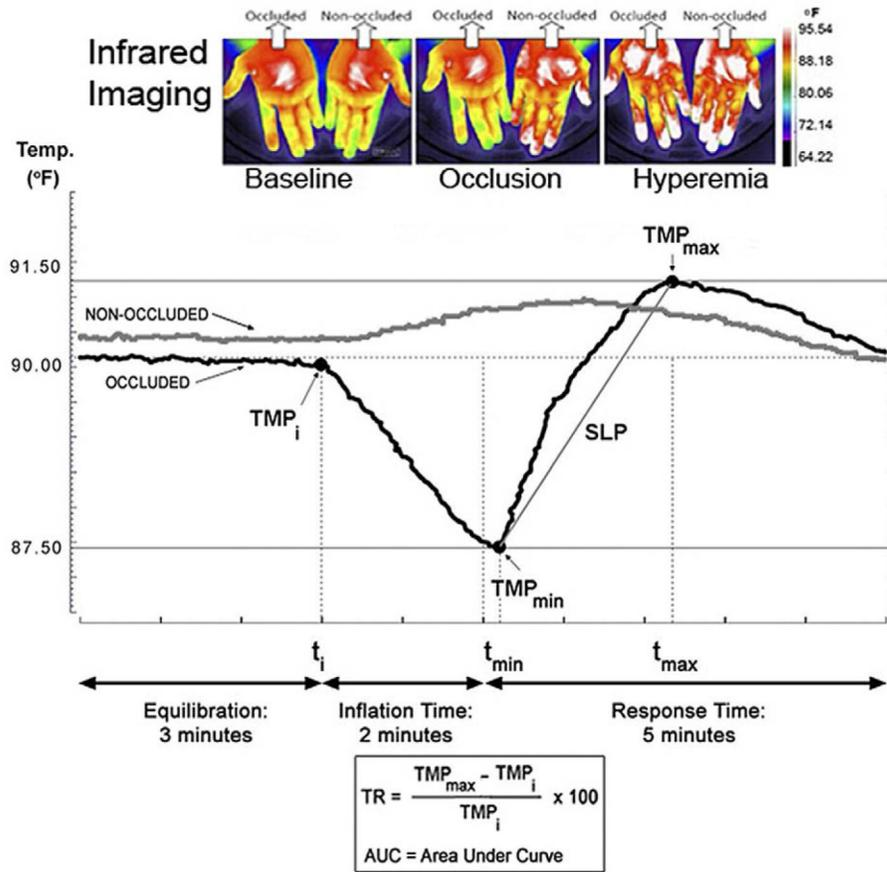
**Figure 1.** Skin temperature changes during cuff-reactive hyperemia, as shown by infrared imaging and digital thermal monitoring (DTM). (SLP, slope.)
